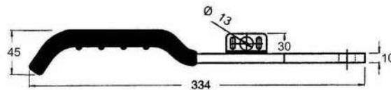
**Art. 38-00066** Maniglia Piatta inox L=334 c/impugn.rivestita *S.s.flat lever with coated grip L=334* (Kg.0,970)
